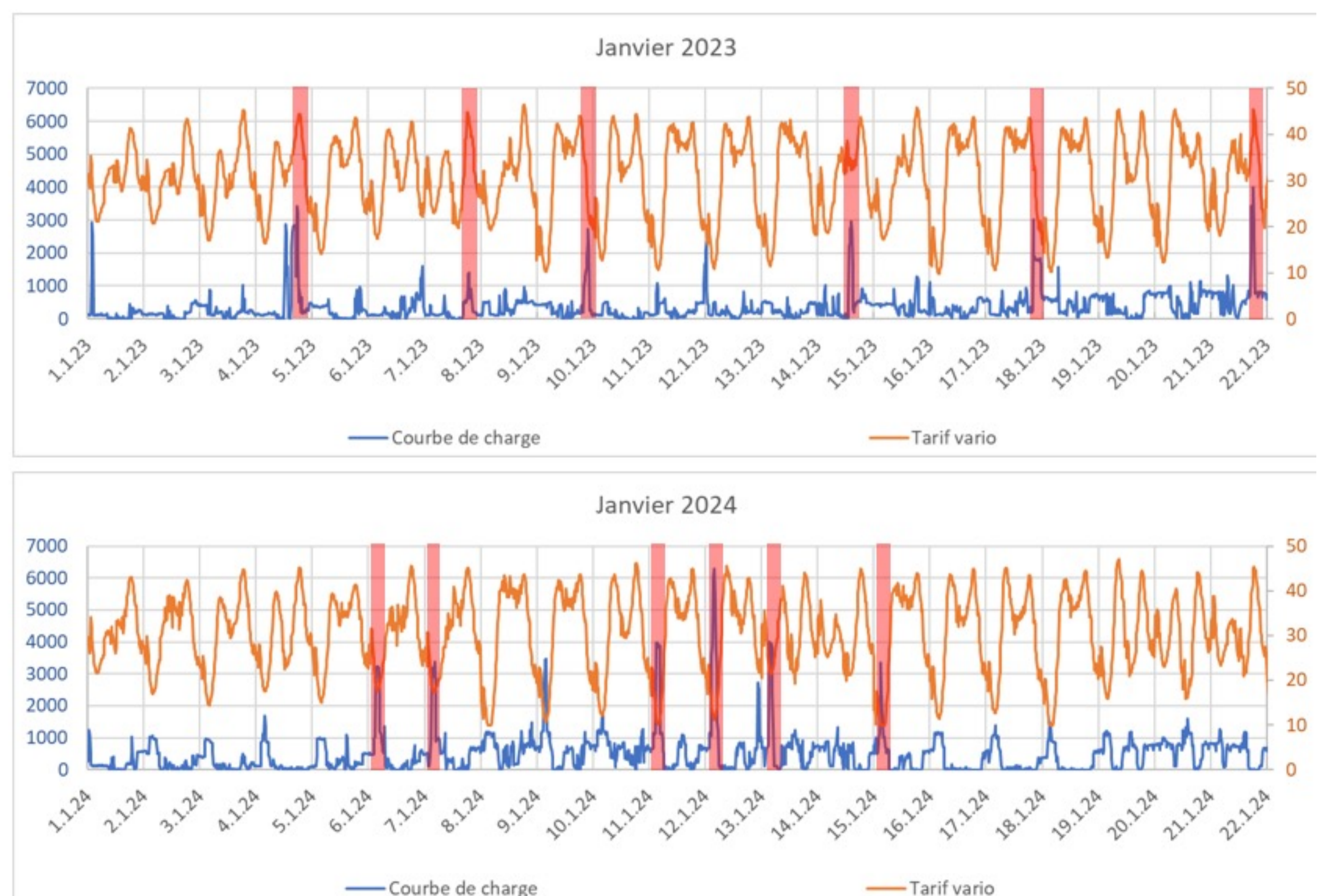
Load of a sample customer without (top) and with Vario tariff (bottom) (pilot)
