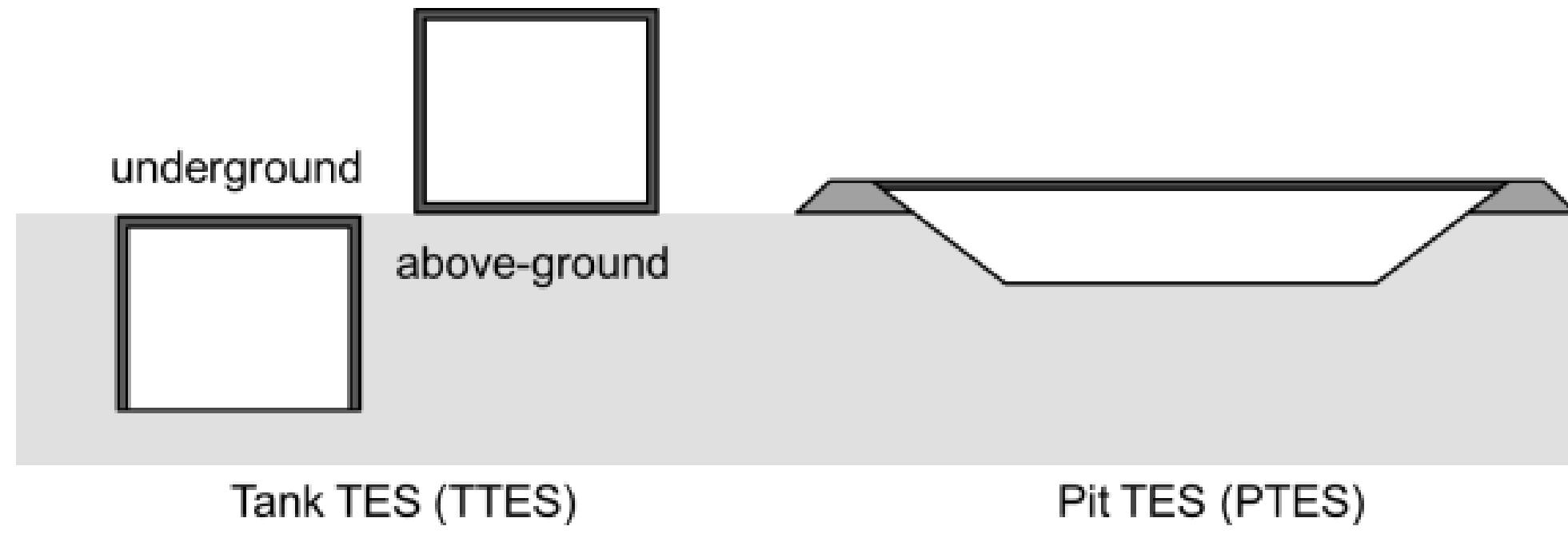
PTES are pits dug in the ground, filled with water and thermally insulated at the top and sometimes on the sides as well. The storage medium is usually water, but can also be in some cases a mix of sand, gravel and water
