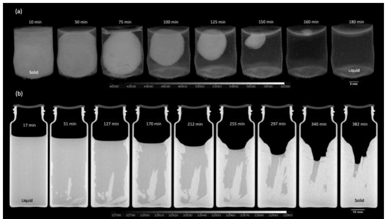
Melting of  $\text{CaCl}_2 \cdot 6\text{H}_2\text{O}$  over time in XCT
