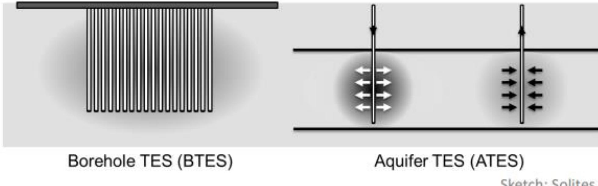
ATES are aquifers directly used to store heat: wells are drilled into an aquifer layer, one for the cold side and one for the warm side. The storage medium is water and ground in the aquifer
