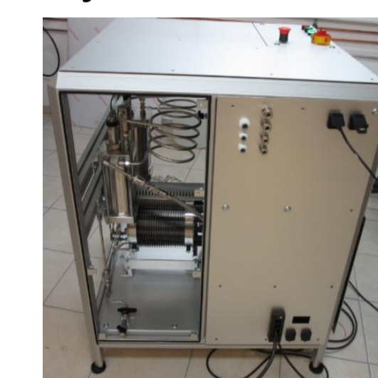
DESL Electrolyzer 5 kW, 20 cells in series
